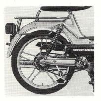
If pedal chain tensioner catches or travels roughly as pedals are operated, realign tensioner so chain travels smoothly.
