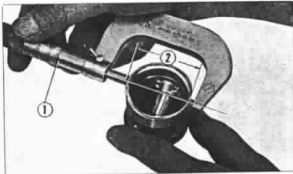
① Micrometer ② Piston diameter Fig. 30
