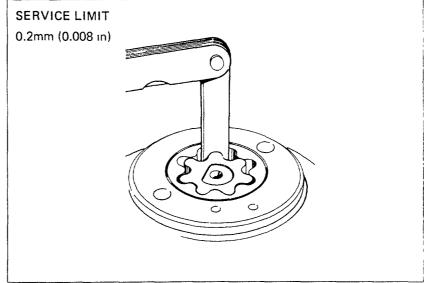
Measure the pump body clearance.
