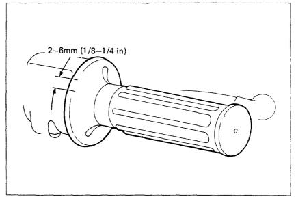
To adjust, turn the adjuster in either direction.
