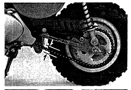
To adjust, loosen the axle nut.
