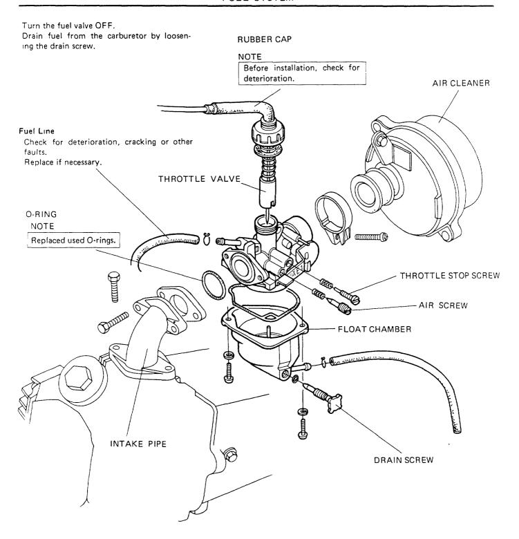
Clean carburetor jets and body with non-flammable or high flash point solvent before installation.
