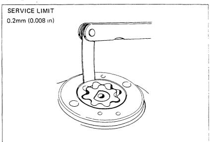
Measure the pump side clearance.
