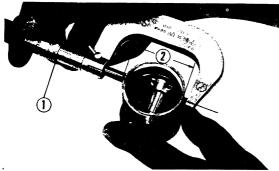
① Micrometer ② Piston diameter Fig. 30
