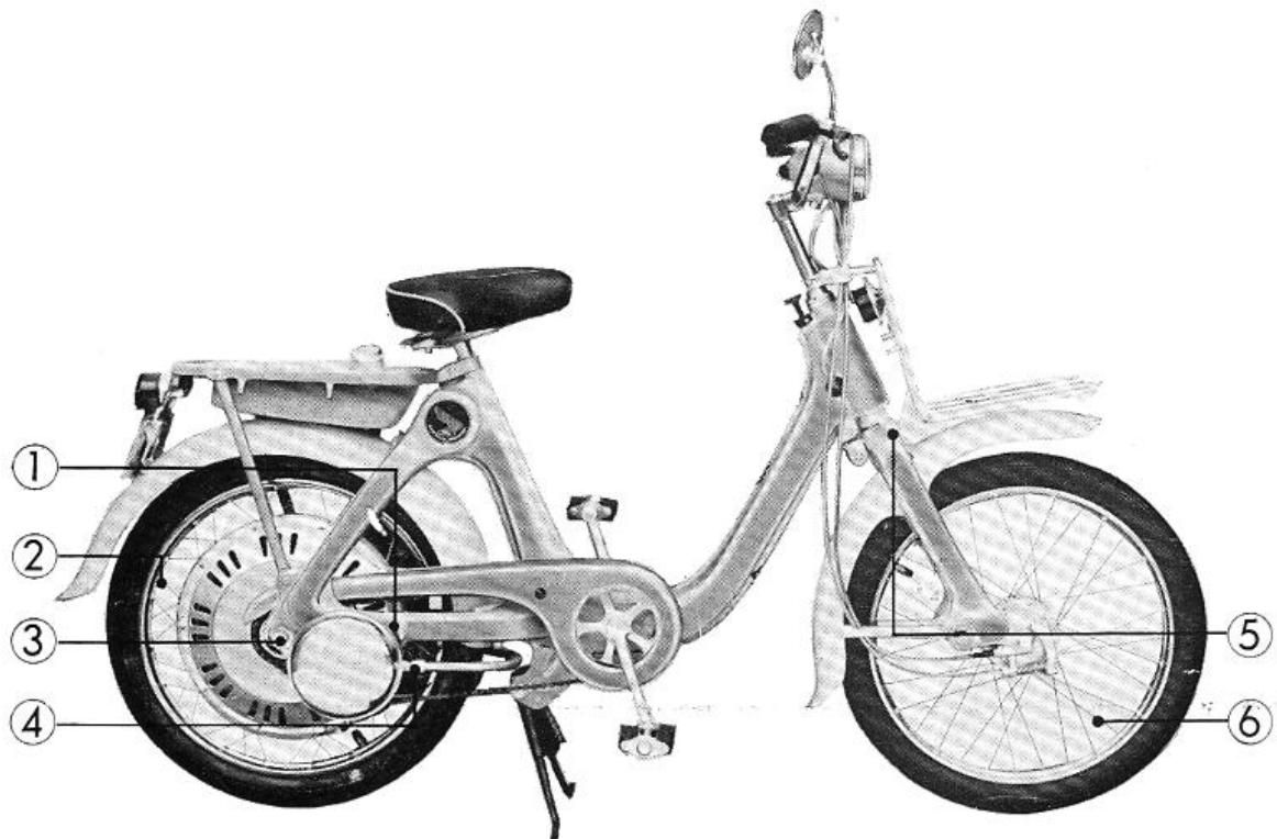
Fig. 1-25 ① 6×14 bolt ② Spoke ③ Rear axle nut ④ Muffler band ⑤ 6×14 screw (2 ea) ⑥ Spoke
